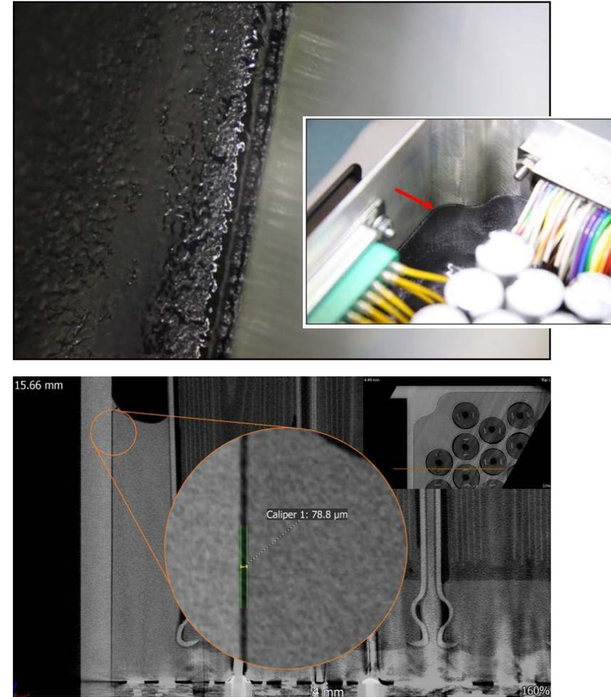
Figure 5- CT scan showing dark line (the crack) between the housing wall and the potting (top of the unit)
