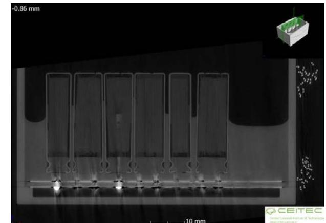
CT scan showing no cracks, no bubbles - EP37 (length side view)
