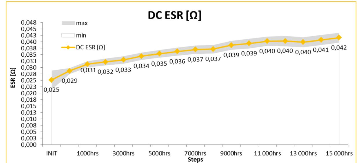
– MTBF determination : after 15 000h of life test without failure, the reliability rate demonstrated is **24 FIT** for one supercapacitor
