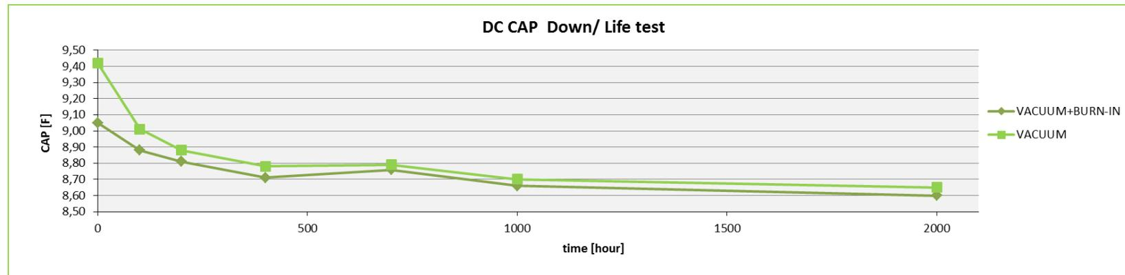
Capacitance degradation for  $50^{\circ}\text{C}$   $0,9 V_{op}$  calendar test condition
